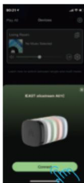
By default, after the factory is powered on and the device is powered on normally, a prompt for network configuration of the new device will pop up after opening IEASTAPP. If there is no prompt, you can press the multi-function button for 6 seconds in WiFi mode (indicator green) and then release it. The device will enter the network configuration mode, and then open IEASTAPP for operation.
